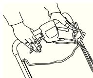
The engine is switched off by moving the stop switch to the stop position.
